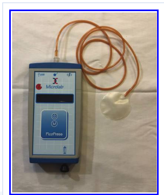
Fig 4. Example of a devices used to measure interface pressure in vivo , PicoPress
