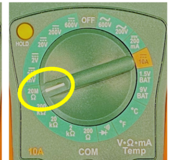
Standard Multimeter Set to Highest Resistance (20 M \Omega )
