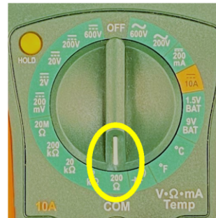
Standard Multimeter Set to Lowest Resistance (200 \Omega )
